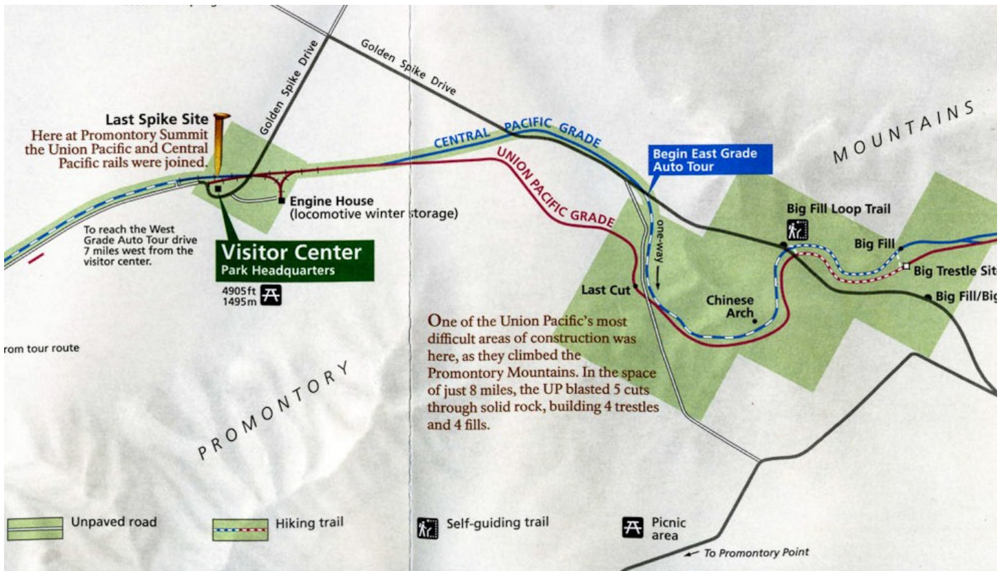
The last few miles of the Union Pacific Railroad as it approaches Promontory Summit. Note the controversial parallel grades. The U.P. did not take advantage of the Central Pacific's "Big Fill", but built a trestle instead.
