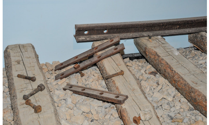
Roughhewn ties, fishplates , rails and spikes used to build the railroad. Rail were 30 feet long and weighed 560 pounds
