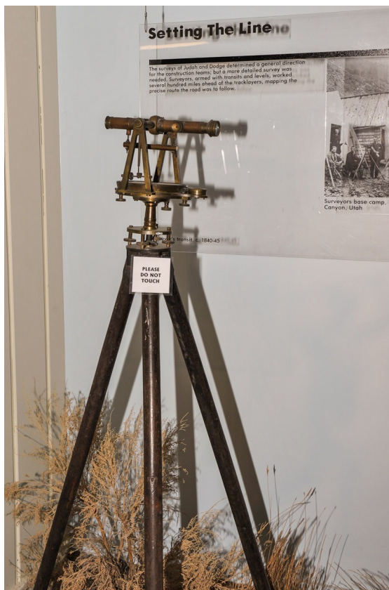
Surveyor's Transit with level bubble. Bearings were taken the compass on the transit plate.
