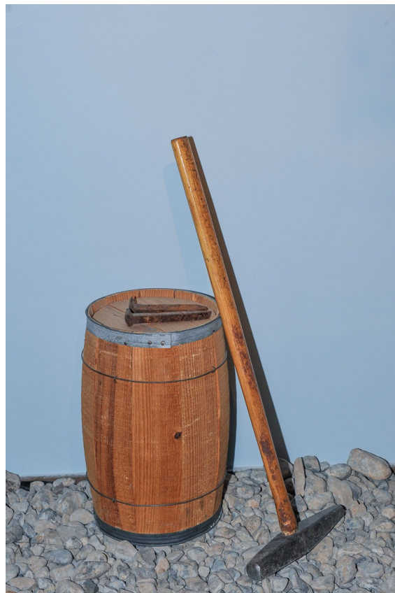
7" iron spikes, blasting powder, and 8 lb. spike hammer. The track layers used three blows per spike to set the rail in place.
